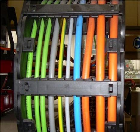
*Vertical dividers used to create cavities*
