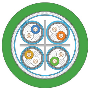
TKFF 390 Cat 7 SF/FTP Ethernet cable for continuous flexing.
